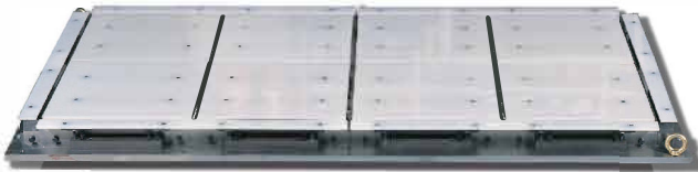
2 cavities by 4 rows for 500x500mm carpet tile
